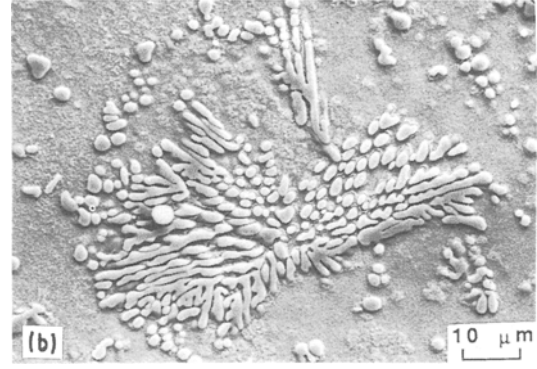
Figure 8 (a–c) A series of secondary electron images at different magnifications showing a discarded microstructure of Cu–30 wt % Co flakes solidified in the drop-tube.
